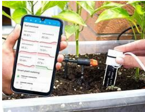
Figure: (5). Representative ESP32-based soil-moisture sensing and automatic watering configuration, adapted from [10].
