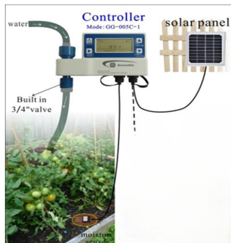
Figure: (4). Representative outdoor solar-powered moisture-sensor irrigation controller, adapted from [9].
