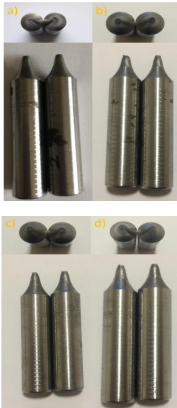
Fig. 20 a) untreated sample, b) P1, c) P2 and d) P3 Photographs of samples after rupture
