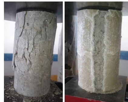
Fig. 8 Failure mode: a) without cover, b) covered by GFRP.
