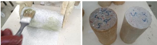
Fig. 5 Covered column with GFRP.
