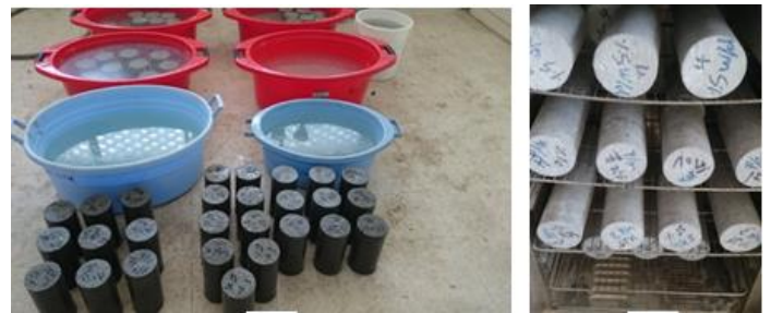
Fig. 4 Curing wet and dry cycle in NaCl (5,10,15% NaCl; in oven of 60°C.
