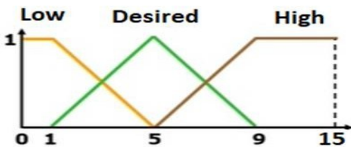
Figure 6: fuzzification of the input water level h(t)
