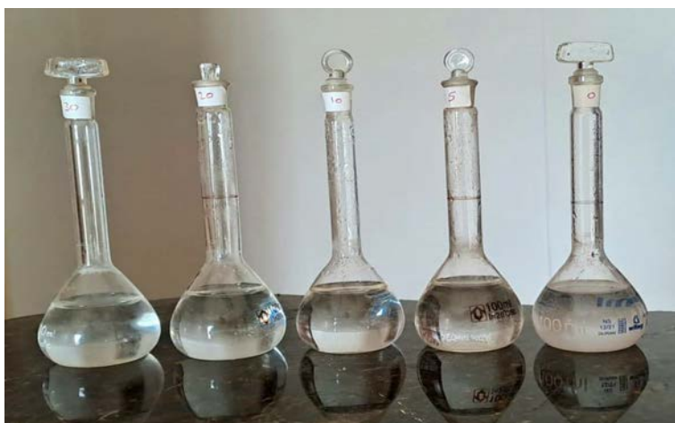
Figure. (3). Scale Test Observation for \text{CaSO}_4 at 70^\circ\text{C}
