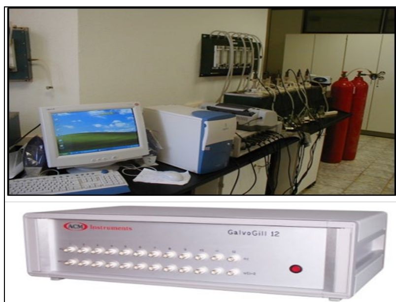
Figure: (1). LPR Gill-12 corrosion test system
