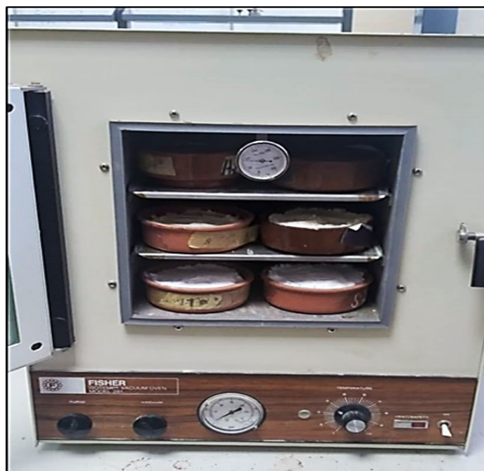
Figure: (2). The electric oven device
